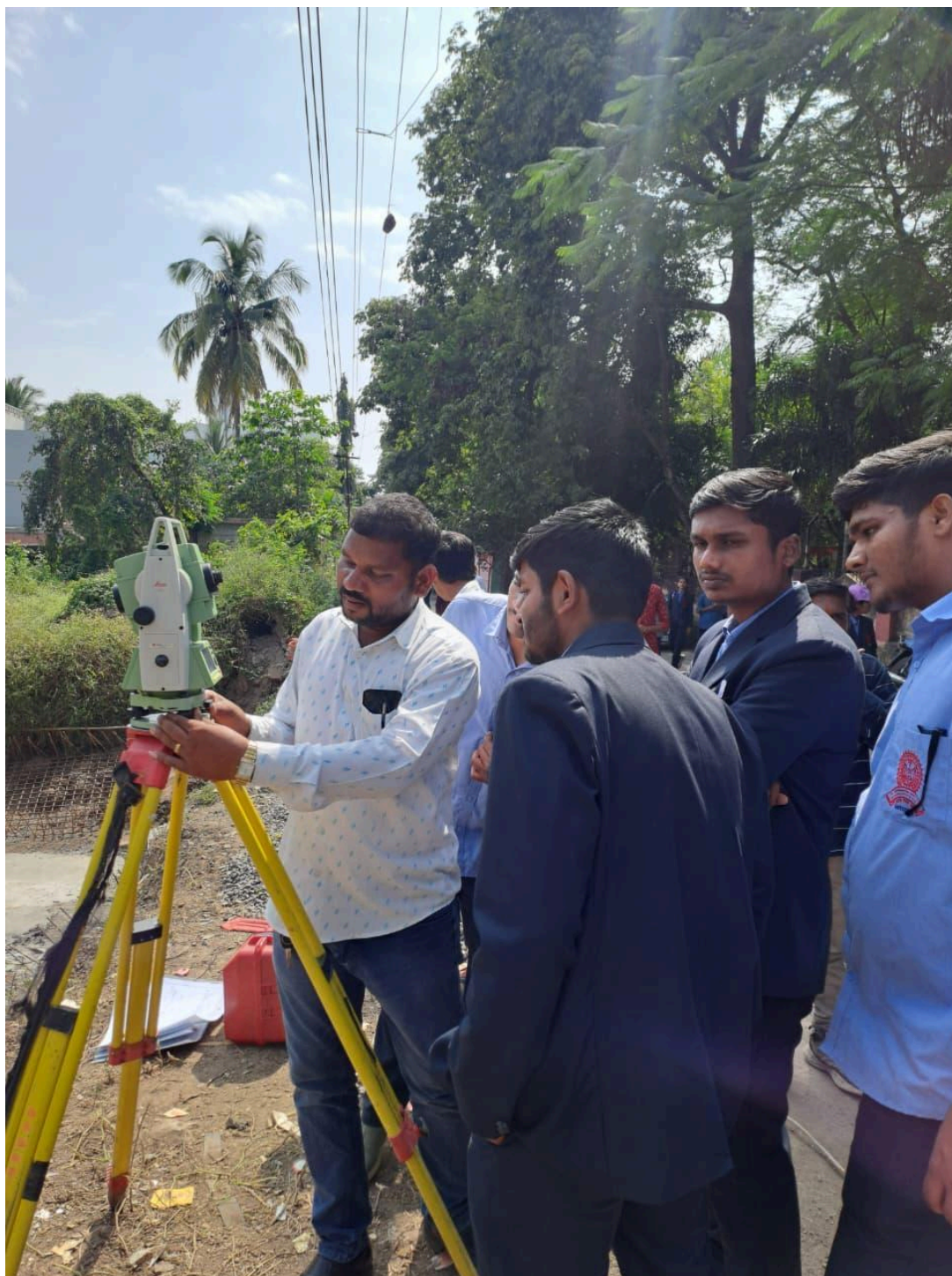
Practical demonstration of Total Station operation as students engage in hands-on learning.
